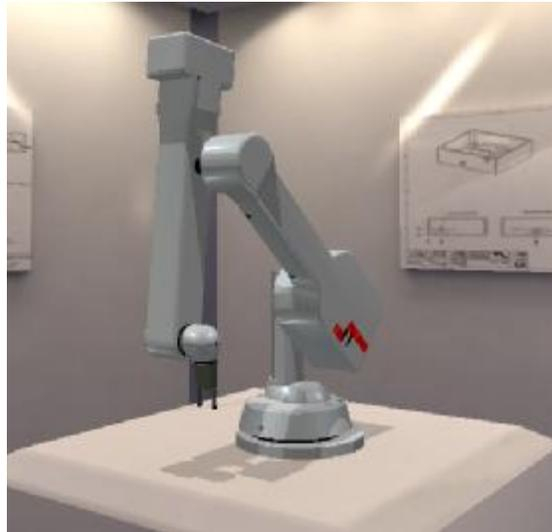
2. Now move the robot sideways using the communication window. Enter 2000 2500 -1000 MOVETO
