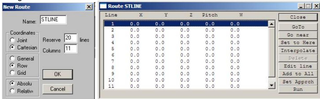
A straight line is merely made up of a number of shorter moves. Each move is itself a slight curve so you need to decide how many segments you require. There will of course be 1 more line than segments. In the above example there are 10 segments, that's 11 lines or columns. If you wanted a much straighter route then pick say 100 segments – 101 columns. In that case you would also need to reserve more lines than 20, say 110. You now see all 11 lines but all are zero.
