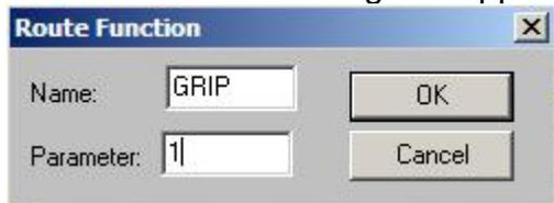
You can also include a delay in the route using MSECS. For example if you want a 5 second delay between lines 4 and 5 then click line 5, click **Insert Func**, enter MSECS in the dialog box and 5000 for the value.
